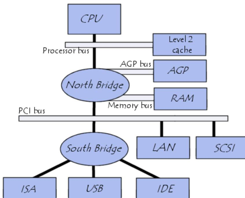
**North Bridge:** It is the connection between the high speed processor bus and the slower AGP & PCI buses. It is responsible for communication from the CPU to memory, the CPU to the PCI (Peripheral Component Interconnect) Express bus, and the Advanced Graphics Port (AGP) device. It is the only motherboard circuit (besides the processor) that runs at the full motherboard speed. It serves as the four way connection between CPU, Memory, Video card and south bridge .
